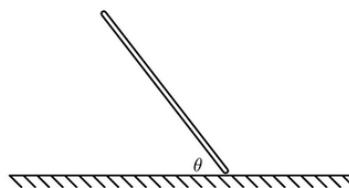
Find a differential equation describing the time evolution of the angle  $\theta$  that the rod makes with the plane, that is valid as long as the endpoint keeps contact with the plane.
