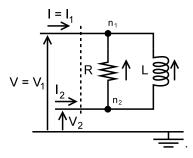
Show that  $I_1 = -I_2$  and eliminate  $I_2$  from the system. Then fix the lower wire to the ground, i.e., impose  $V_2 = 0$ , and eliminate  $V_2$  and  $n_2$  form the system, so that with the definitions
