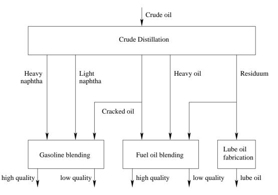
Crude oil is transformed by a number of distillation processes into different kinds of oil, which is then blended into different kinds of marketable products.
